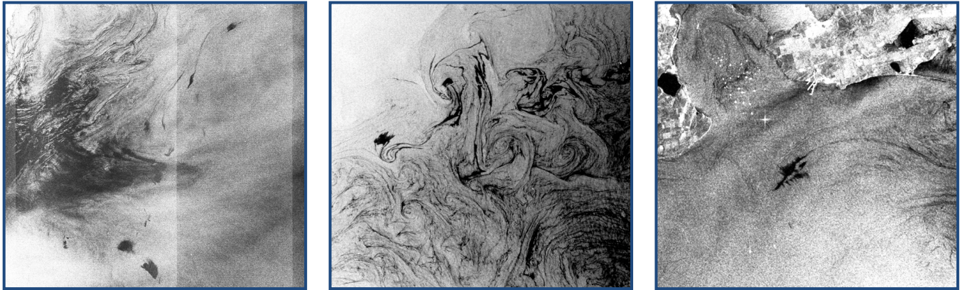
Fig. 1. Slicks due to algal bloom as seen in ASAR Envisat imagery: (a) subscene (150x150 km) of the ASAR Envisat image collected on 03.07.10 at 17:52 UTC in the western part of the Black Sea; (b) subscene (100x100 km) of the ASAR Envisat image collected on 18.09.10 at 19:32 UTC in the southern part of the Black Sea; (c) subscene (50x50 km), of the ASAR Envisat image collected on 09.06.09 at 07:50 UTC in the north-eastern part of the Black Sea near the Kerch strait
