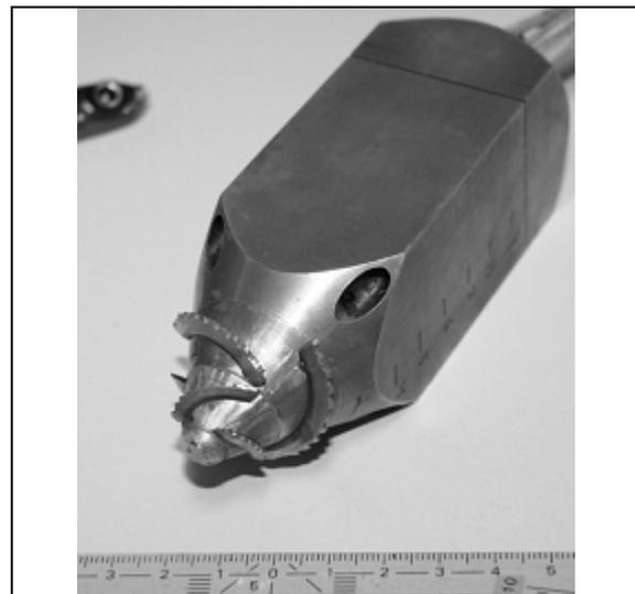
Fig. 2 The cross-section of the thermal drill prototype is 40mm x 40mm. Its final length will depend on the integrated payload.
