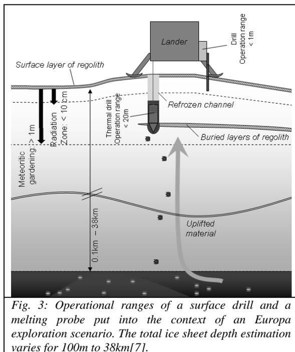
The coming step in this development will be tests of this system in a cyro-vacuum-chamber to evaluate its performance in sublimation environment. This will then be followed by a study of possible instrument payloads, which such a system could carry into the ices of Jupiter moon Europa.
