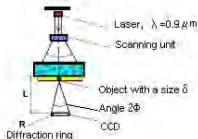
Fig. 1 The diffraction camera scheme
