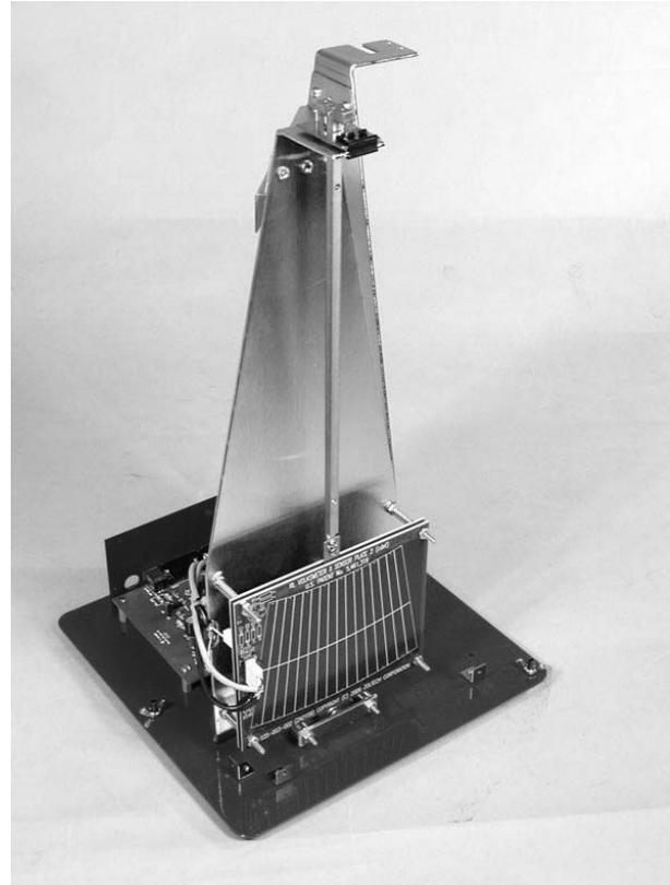
Figure 5. A Commercial capacitive-sensing tiltmeter, also able to achieve nanoradian precision.
