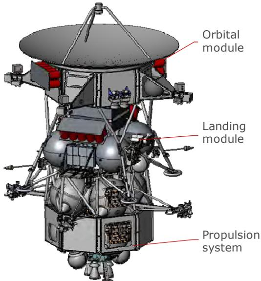
The orbital module is the basic structural element of the space vehicle and provides the control of the SC at all stages of flight. At the orbit around Europa it serves for research experiments and relaying.
