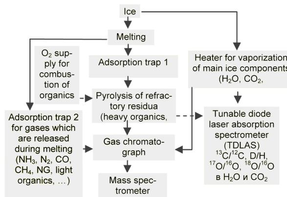
Fig. 1. General scheme of the gas analytic package for the Europa lander.
