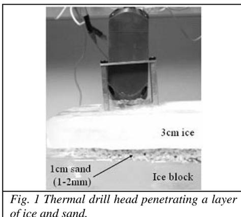
Fig. 1 Thermal drill head penetrating a layer of ice and sand.
