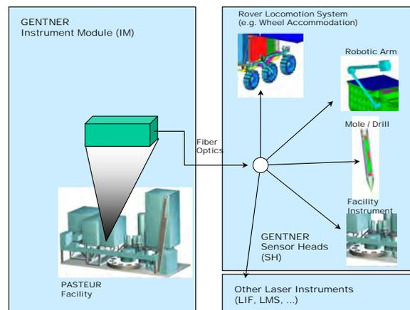
**Figure 1:** Schematic of the GENTNER instrument as originally proposed<sup>4</sup> for ESA’s Mars payload Pasteur. It easily can be adapted to the *in-situ* operation on Europa’s surface and to various lander designs.
