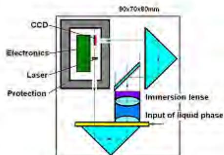
Fig. 2. The principle scheme of the instrument
