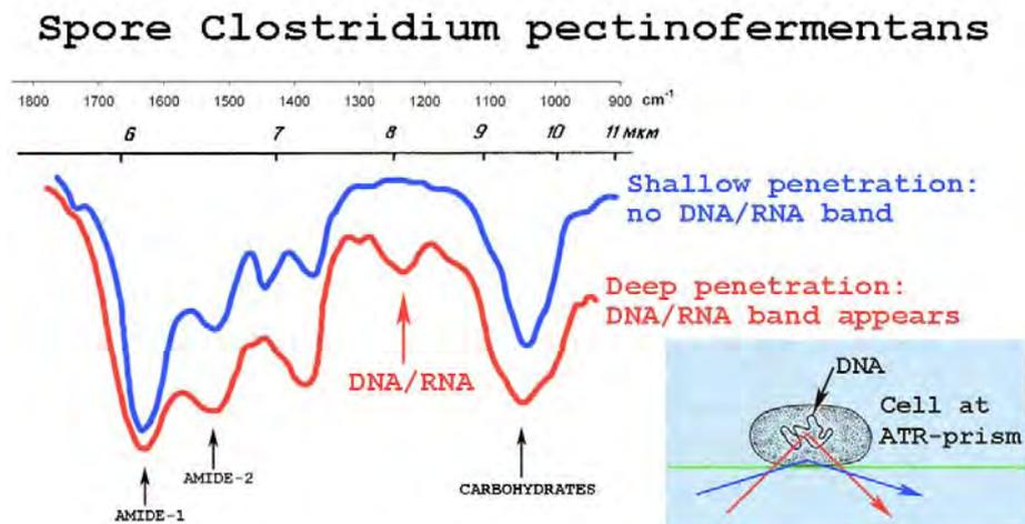
Fig. 1. Bio-molecules have characteristic IR bands, e.g. all proteins show «Amide-1» & «Amide-2» bands. Different AIO inside ATR-prism provides sampling depth varying.
