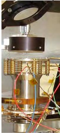
Figure 1. Laser ablation mass spectrometer
