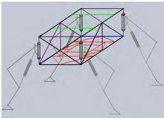
Figure1: Line diagram of SCOUT-ETL, with landing gears and dampers.
