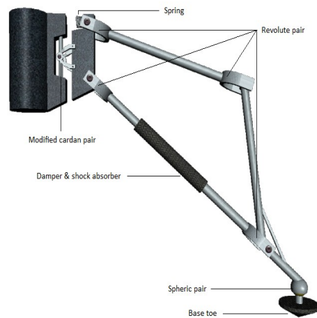
Figure5: Equivalent mechanism [Landing gear]
