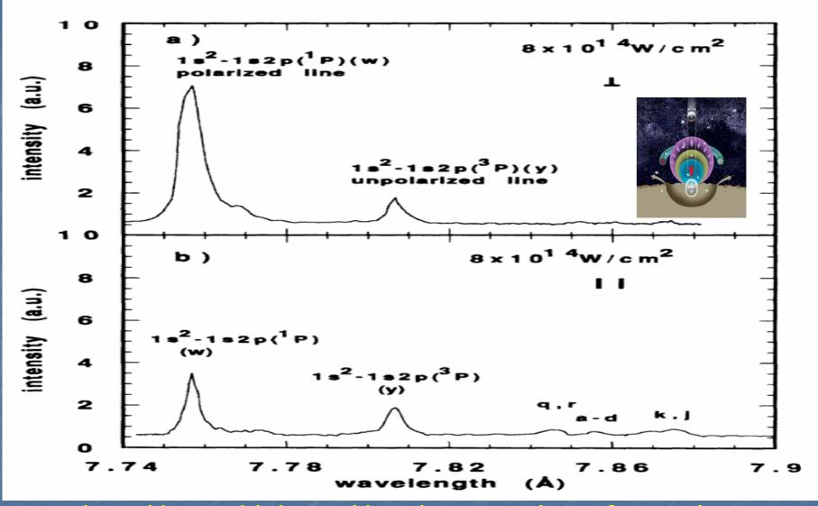
Helium-like and lithium-like aluminum lines from a laserproduced plasma. The polarization components are resolved. (T. Fujimoto, E.O. Baronova, and A. Iwamae)
