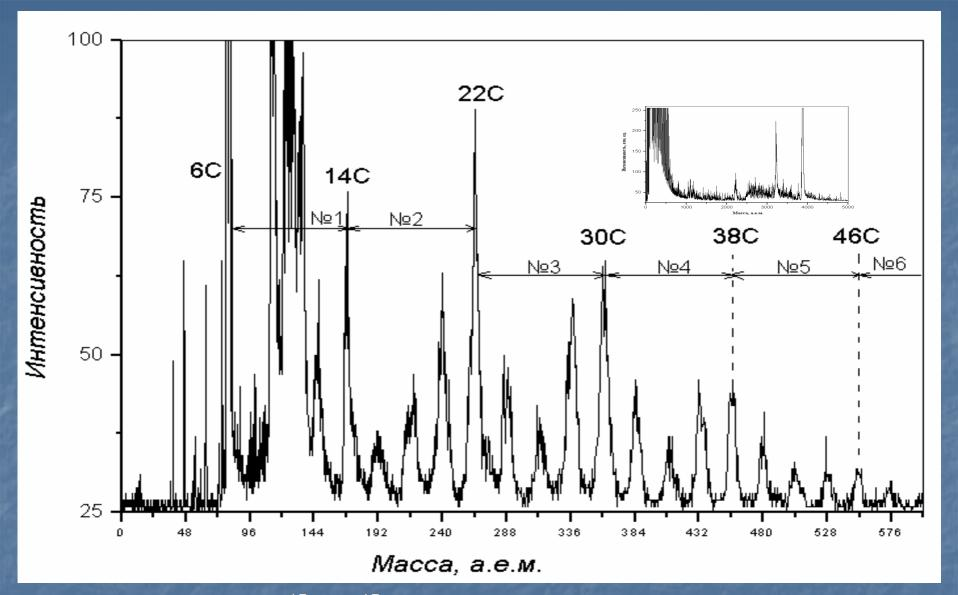
Spectrum of carbon and <sup>15</sup>NH<sub>4</sub> <sup>15</sup>NO<sub>3</sub> mix, received at laser radiation spot diameter ~1,5-2MM. The mass peaks (in region Nº 1-6) was interpreted as branched polymer OC and cycle-alkenes (C<sub>8</sub>) based on linear acetylenic carbon ( $-C_2-C_2-$ ) or the «sp» carbon allotrope. (Fragment of spectrum).
