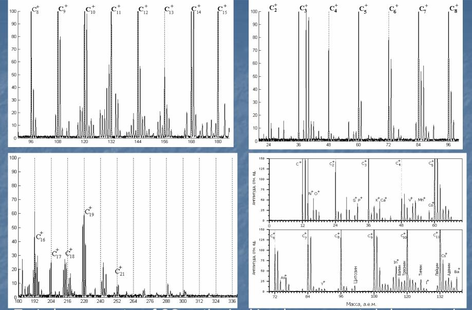
Typical mass spectra of OC synthesized in a laser-generated plasma torch under the action on pure carbon and its mechanical mix of NH<sub>4</sub>NO<sub>3</sub> for the spot diameter ~50mkm and pulse duration ~1ns. In similar spectra were identified 11 amino asides and carbines. The most important properties of living matter have appeared at pre-biological stage of the evolution of a life in the physical and chemical processes.
