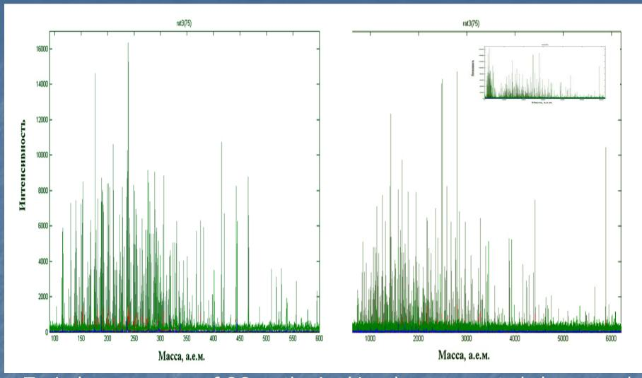
Typical mass spectra of OC synthesized in a laser-generated plasma torch under the action on pure carbon and its mechanical mix of  $(NH_4)_2HPO_4$  for the spot diameter ~50mkm and pulse duration ~1ns. According to preliminary interpretation observed mass peaks may contain nucleotides (left) and its oligomers (right)
