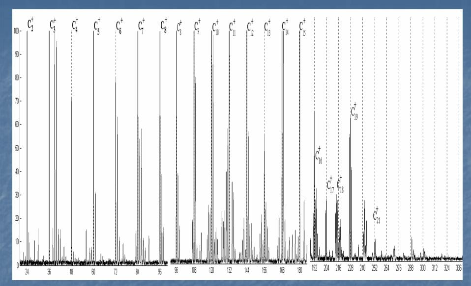
Typical mass spectra of OC synthesized in a laser-generated plasma torch under the action on pure carbon and its mechanical mix of  $NH_4NO_3$  for the spot diameter ~50mkm and pulse duration ~1ns. In similar spectra were identified 11 amino acides and carbines.
