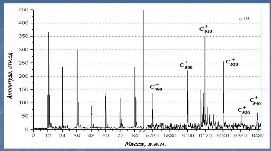
Fragments of mass spectrum of the **giant fullerenes**. Typical spectra of carbon and hydrocarbon structures were obtained with the  $d_L \sim 2 \text{ mm}$  and  $W_L \sim 10^9 \text{ W cm}^{-2}$ . Mass peaks containing from 480 to 540 C atoms correspond to the typical mass of "onion"-like fullerenes, representing enclosed each into other quasi-spheres, with following quantities of C: 60, 240, 540, 960... Mass peaks at 12-96 a.m.u. represent carbon and hydrocarbon ion-radicals.
