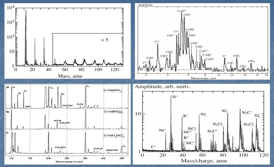
Typical mass spectra of OC synthesized in a laser-generated plasma torch under the action on pure carbon and its mechanical mix of different elements and salts the diameter of spot is ~50mkm (their compositions are given on each mass spectra) and pulse duration ~10ns.
