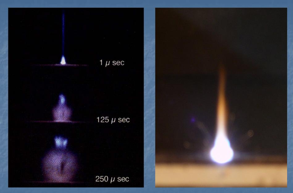
The plasma torches generated under the influence of SHVI (left) and the laser radiation (right) are identical.
