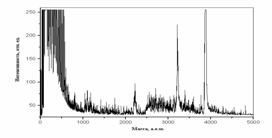
Spectrum of carbon and <sup>15</sup>NH<sub>4</sub><sup>15</sup>NO<sub>3</sub>, mix received at laser radiation spot diameter 1,5-2мм. The mass peaks 2250, 3250, 3900 a.m.u. was interpreted as dendritic type, hyperbranched polymer OC, mass peaks in regions 1000-2000 and 2500-3100 a.m.u.- as peptides. (A full spectrum).
