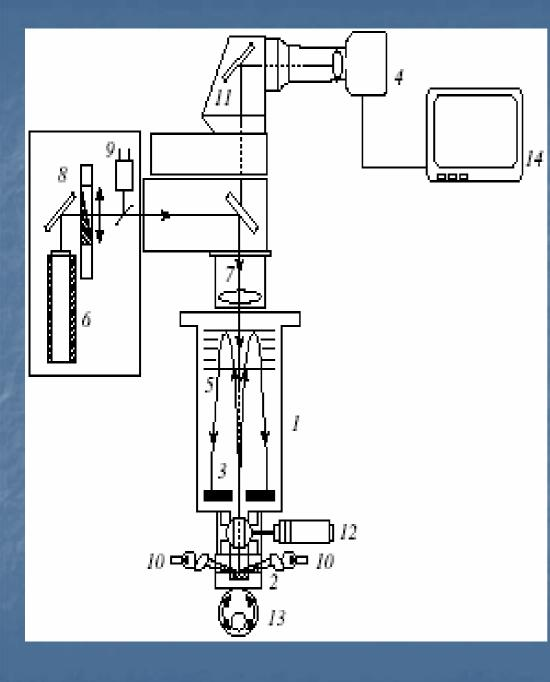
A scheme of the LASMA- TOF laser mass-reflectron: 1—vacuum chamber, 2—interchangeable carriage with sample, 3-detector, 4—TV camera, 5—reflector, 6—laser, 7-focusing lenses, 8-neutral filter, 9—radiation power meter, 10-target illuminator, 11-microscope, 12-motorized vacuum valve, 13—carriage adjusting system, 14—monitor.
