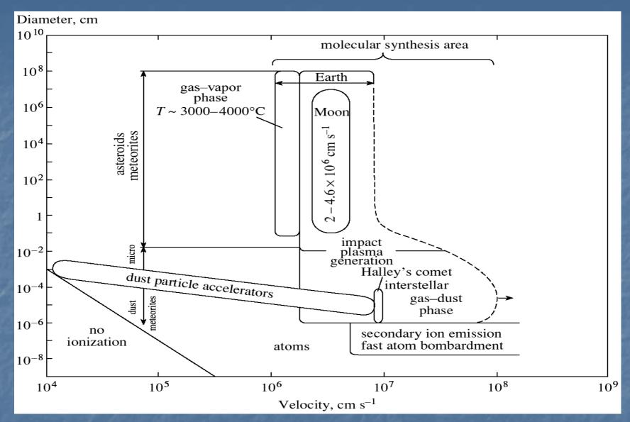
The overall picture of impact plasma generation in various processes in nature and in a laboratory as a function of the body size and velocity
