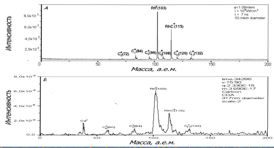
Comparison of mass spectra from laser modeling of SHVI and ones obtained in the dustimpact experiments. Spectra were obtained: (a) under the impact of laser radiation on the target made of the pure C and Rh mechanical mixture (b) in dust-impact experiments using the dust particle accelerator with the impact of carbon particles on the pure Rh target.
