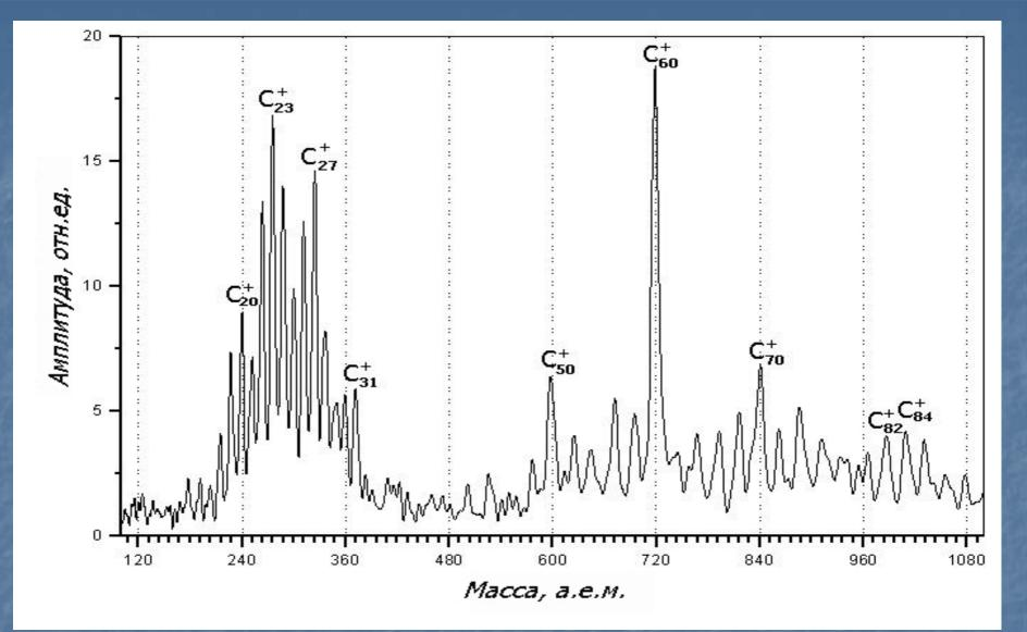
Mass spectrum of the fullerenes and their fragments. The spectrum obtained in laboratory experiments with  $d_{L} \sim 2 \text{ mm}$  and  $W_{L} \sim 10^{9} \text{ W cm}^{-2}$ . Peaks corresponding to the masses from 19 to 31C with a step 1C with high probability may be referred to the individual fragments of the fullerenes, as well as 50, 60, 70 and 82-84C mass peaks with a step 2C– to the fullerenes itself.
