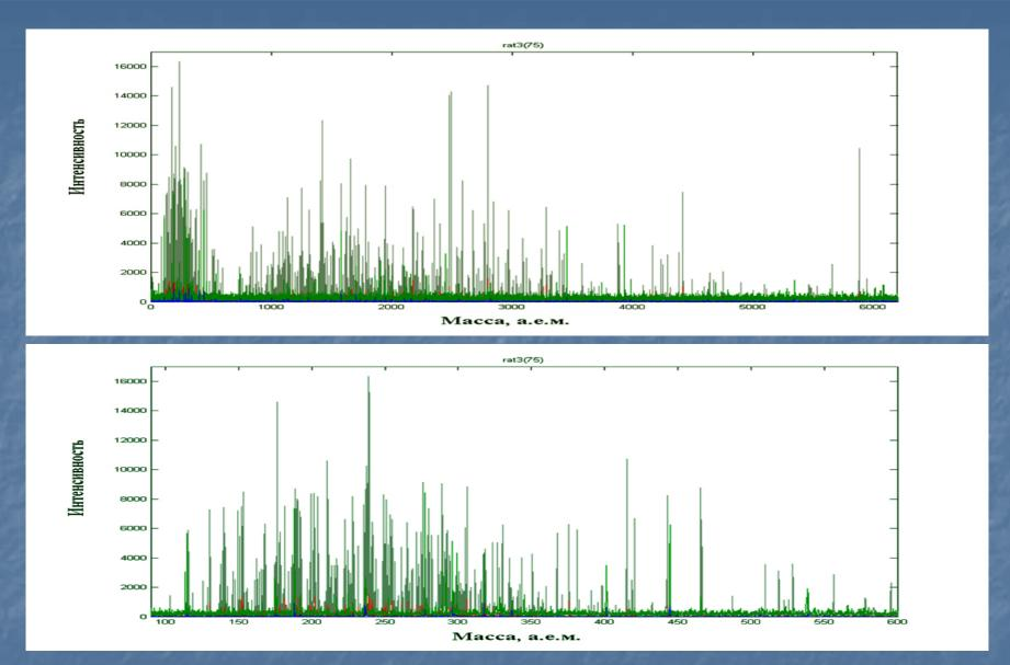
The spectrum and it fragment of a mix carbon and  $(NH_4)_2HPO_4$  for diameter of spot ~ 100 mcm.
