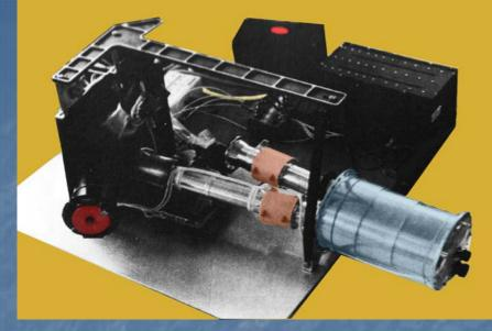
LIMA was also planned for the mass and isotopic composition measurements of Phobos regolith. It was planned to deliver the sample to the spacecraft by harpoons in the framework at first version of closed Soviet project Phobos.
