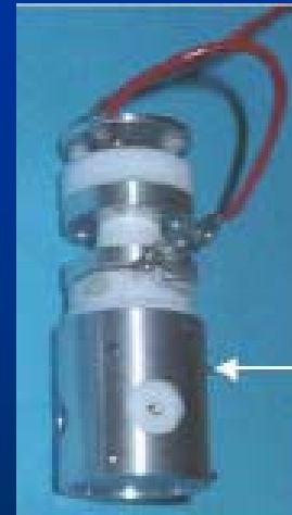
Prototype, ruggedized ion trap mass-spectrometer Open University (Rosetta)
