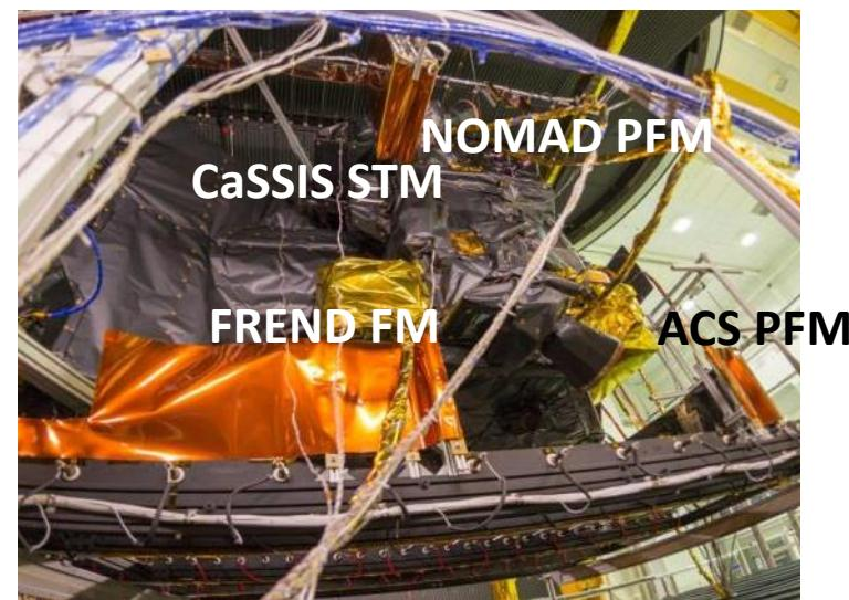
TGO Instruments onto S/C in TV Chamber
