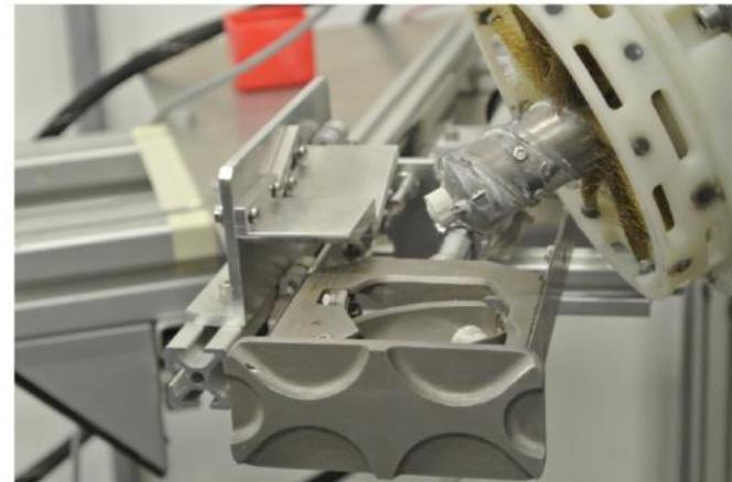
Sample Deposit into Core Sample Transportation Mechanism by Drill
