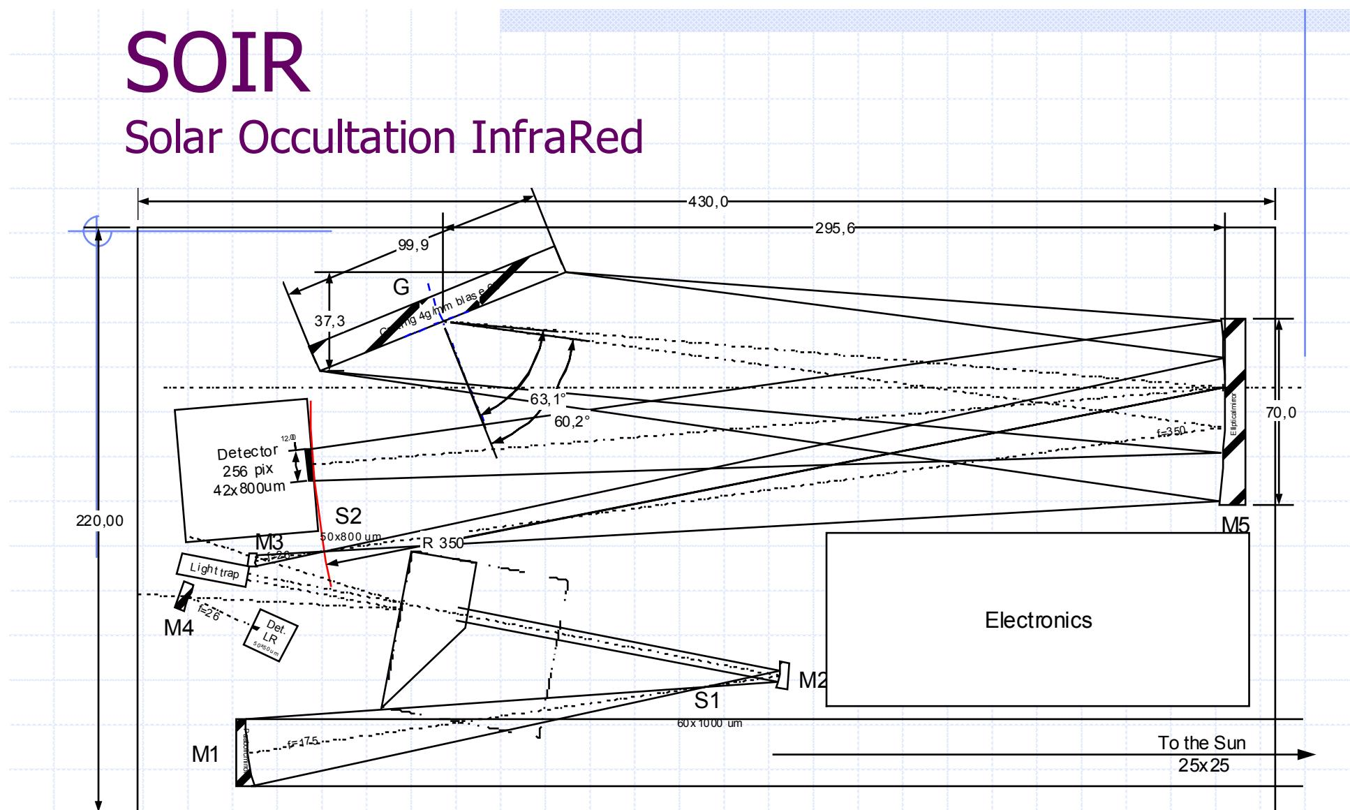
Figure 3. Layout of the high-resolution solar occultation spectrometer. M1 (off-axis parab.  $f=175$ ) – entrance telescope; S1 – field diaphragm; AOTF; M2, M3, M4 ( $f=26$ ) – AOTF collimator; light trap; LR detector; S2 – HR spectrometer slit; M5 (off-ax. parab.,  $f=350$ ) – HR spectrometer collimator; G – HR spectrometer grating; HR detector.
