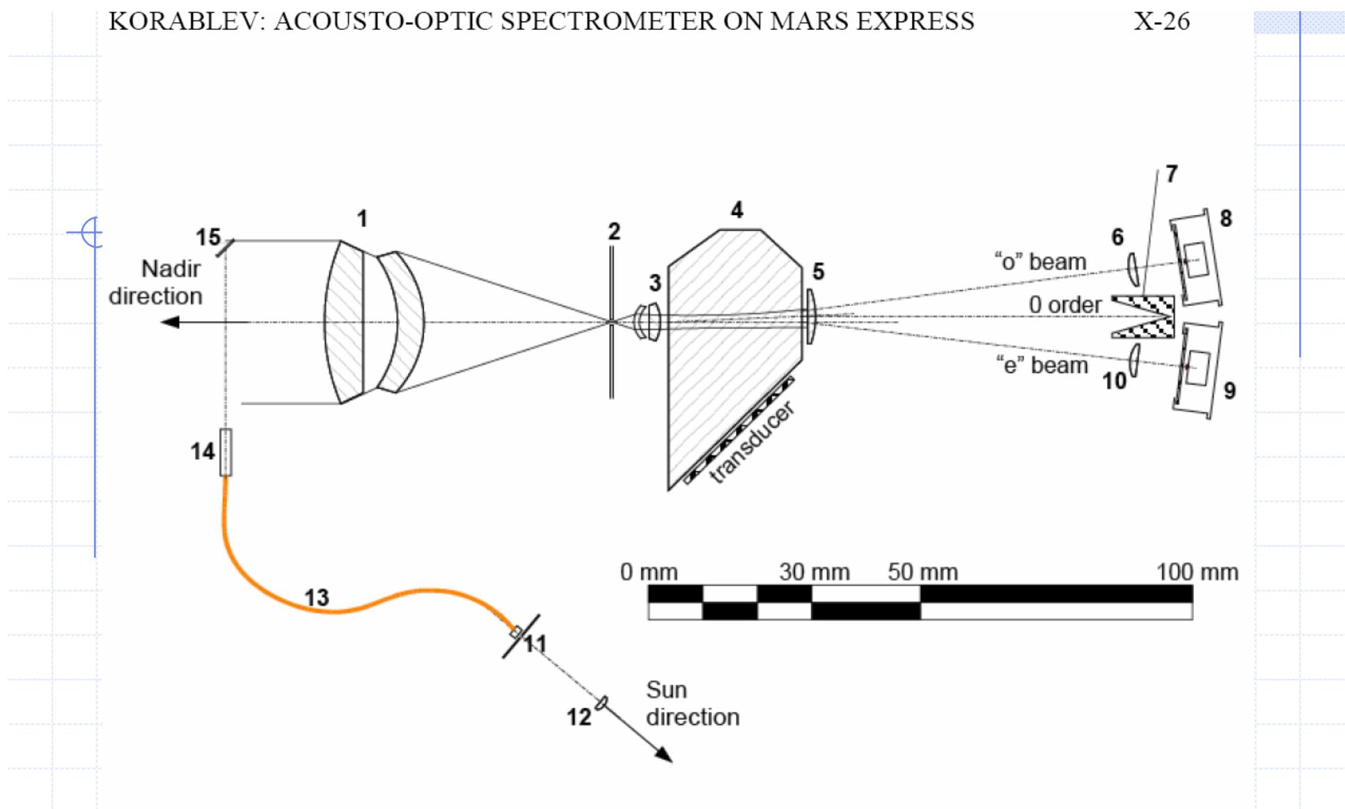
Figure 1. Optical scheme of the IR spectrometer. 1- front-end telescope objective; 2- FOV diaphragm; 3, 5 - collimator; 4- AOTF crystal with actuator; 6, 10- detector proximity lenses; 7 – zero order light trap; 8- detector “1” (ordinary), 9 – detector “2” (extraordinary); 11 – Sun aperture entry lens; 12 – Sun FOV diaphragm; 13- optical fiber; 14- collimating gradient lens; 15 – Sun entry folding mirror.
