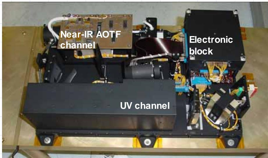
SPICAM – versatile atmospheric spectrometer
